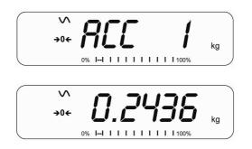
• When the scale is at zero place a second weight. Press [Print] to accumulate the weight. Remove the weight and press [Print]. The display will show "ACC 2" for 2 seconds and then show the new total.
